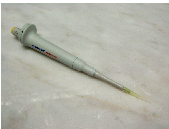
Figure 1- Eppendorf fixed micropipette of 100 \mu\text{L}
