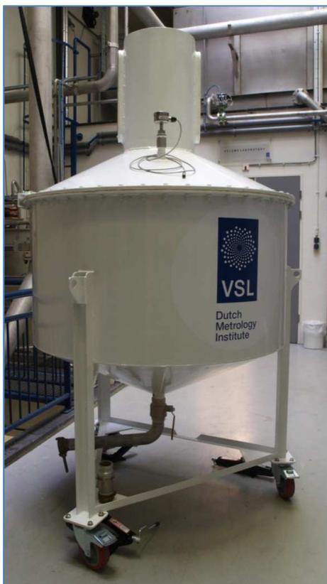
**Figure 1** – proving tank of 1000 L
